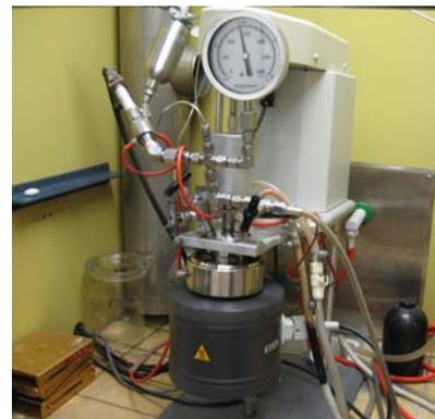
Figure 2: Batch reactor
