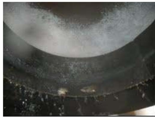
Fig. 3. Water-air vortex layer.
