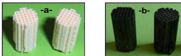
Fig 1. The as-received monoliths (1 cm in diameter) (a) and the catalysts after wash-coating by porous alumina and impregnation by iridium (b).
