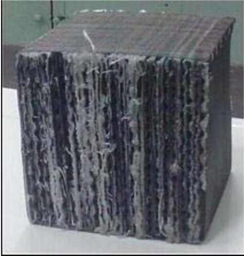
Fig. 2. External view of the catalytic cartridge with glass-fiber catalyst.
