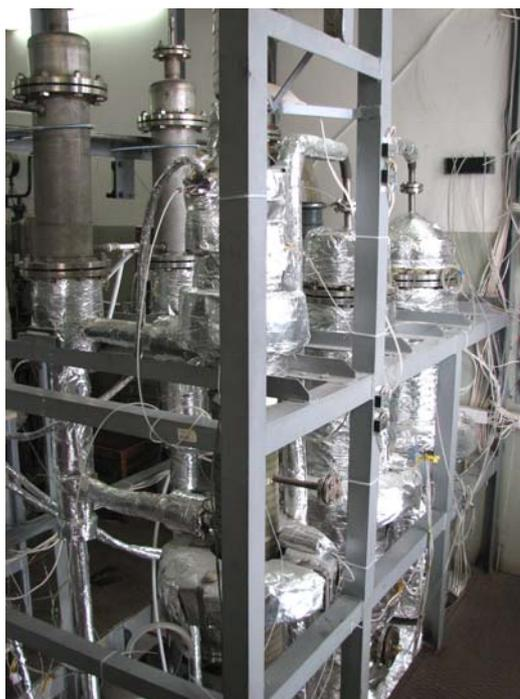
and-tube heat exchangers cooled by cooling water at the first stage and by antifreeze at the second one. The plant is equipped by a chilling machine. Condensate from two separators is collected in an accumulating vessel. The plant is fully automated and controlled by PC. Methanol and product flowrates are measured by electronic balances. Gas composition analysis is performed by GC connected to five points along a technological scheme by heated lines and is fully automated and controlled by PC.
