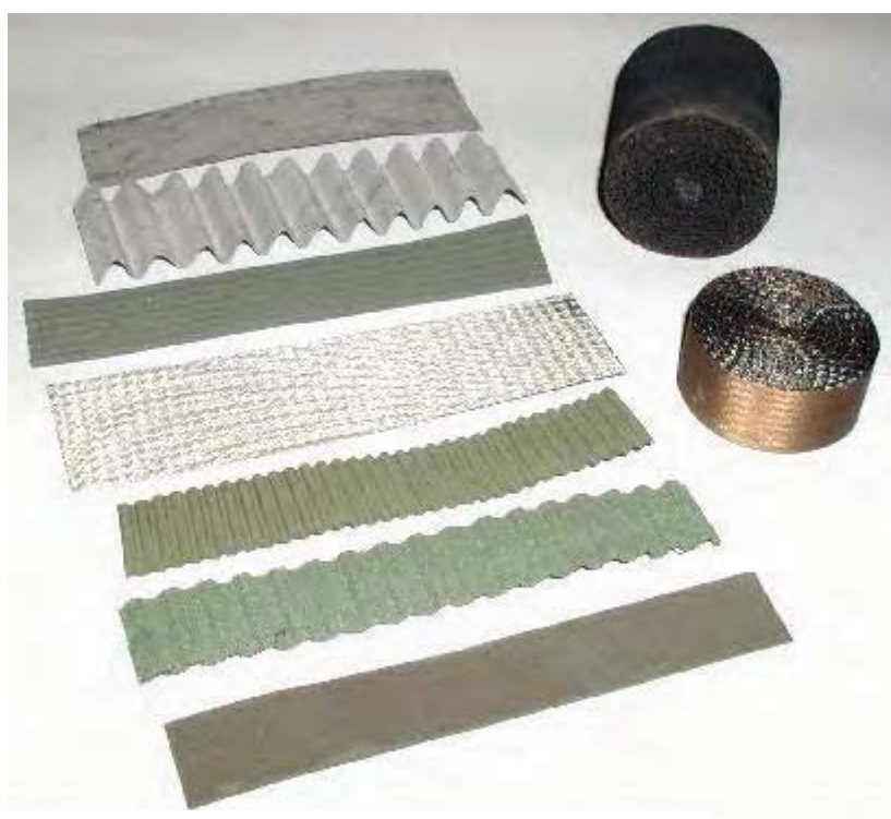
Fig. 1. General view of catalytic strips and monolith reinforced metal porous catalysts.
