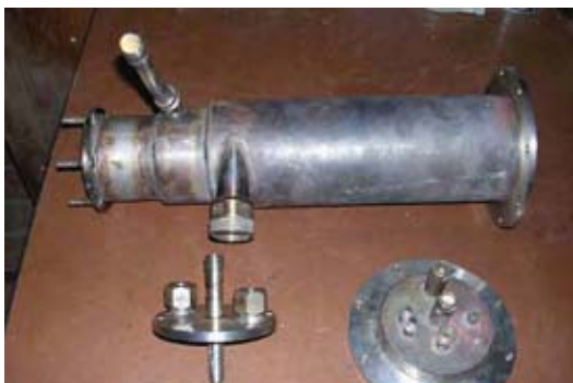
Fig. 2. A general view of the reactor with in-built heat exchanger
