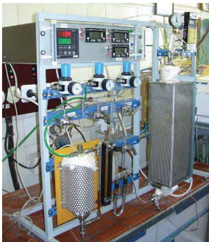
Fig. 1. General view of experimental set-up with fix-bed flow catalytic reactor for vegetable oil feed stock hydrogenation.
