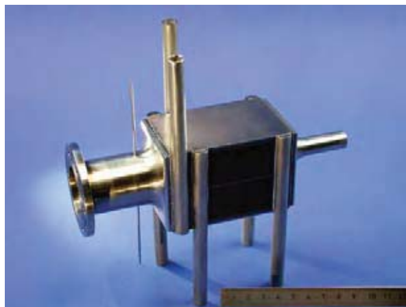
Fig. 4: Integrated catalytic steam reformer afterburner for diesel fuel developed at IMM
