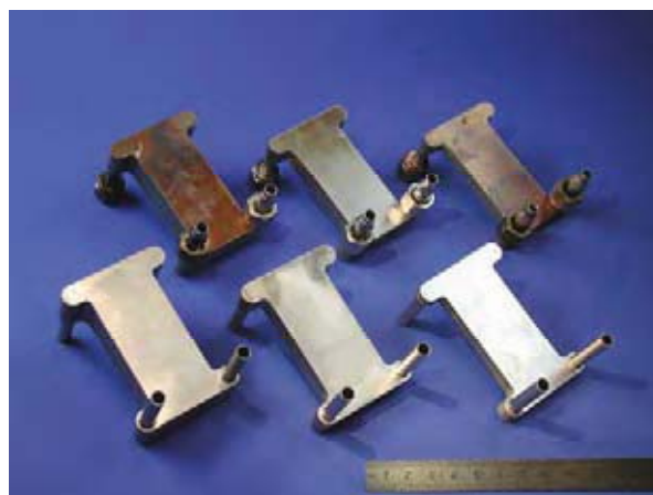
Fig.2: Micro-structured heat-exchangers joined by brazing
