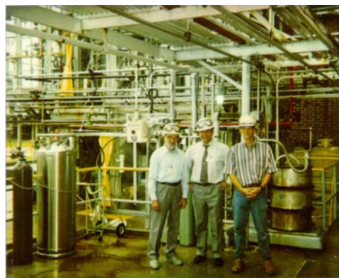
Pilot plant for synthesis of phenol from benzene, with nitrous oxide used as the oxidant (ALPHOX, USA)
